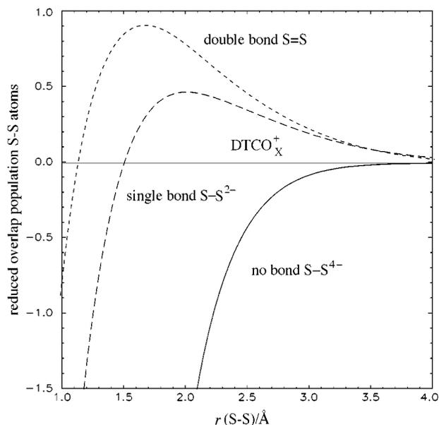
**Fig. 3** Reduced overlap population between S atoms vs. S–S distance in S<sub>2</sub>, S<sub>2</sub><sup>2-</sup>, S<sub>2</sub><sup>4-</sup>, and DTCO<sup>+</sup>.
