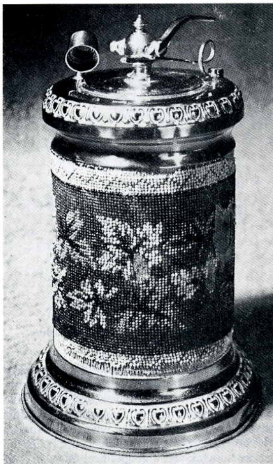
Figure 2. Döbereiner lighter, from the collection of the Kirms-Krackow House in Weimar, Germany.
