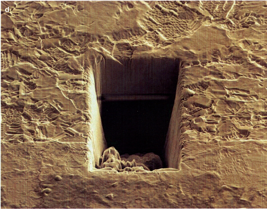
(d) In a multilayer material formed of copper, silicon oxide and silicon, a focused ion beam has milled a 10 \times 20 \times 14 -micrometer trench that casts realistic shadows in the “light” from a scanning electron microscope. (Experiment by G. C. Gazzadi and S. Frabboni.)
